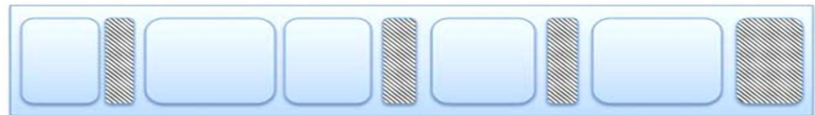
Fragmented memory before compaction
